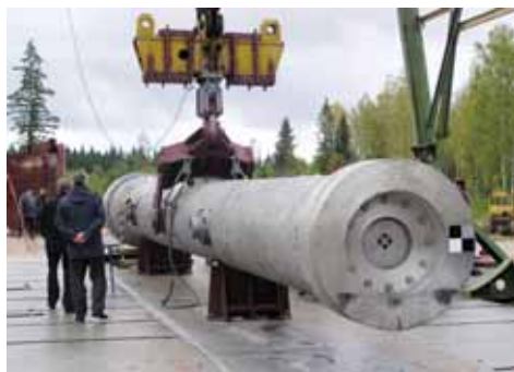
ТУК на испытаниях на полигоне ОКБМ / TUK under testing at the proving ground of Pilot Machine-building Construction Bureau
